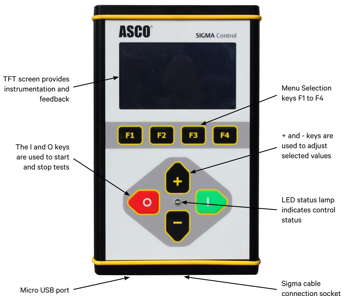
Figure 1-4 The Dynamometer Hand-held.
