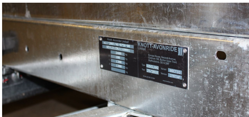
Figure 2-2 Trailer rating plate
